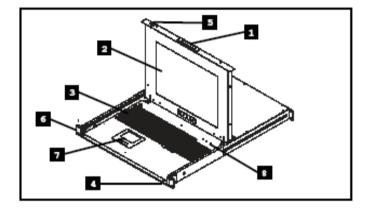
1. Handle: Pull to slide the module out; push to slide the module in.
